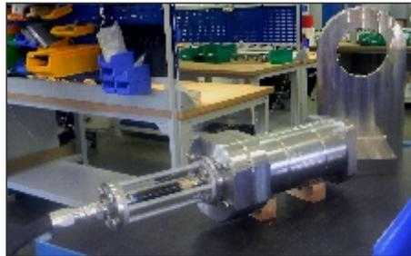
rotation arm was also designed to fit the specific shackle model specified by the customer. Because it would be used in an oil and gas application, ABS witnessing of proof load and calibration was required, along with a certificate of conformity, 3.1 materials certificate and manufacturers certificate of origin.
